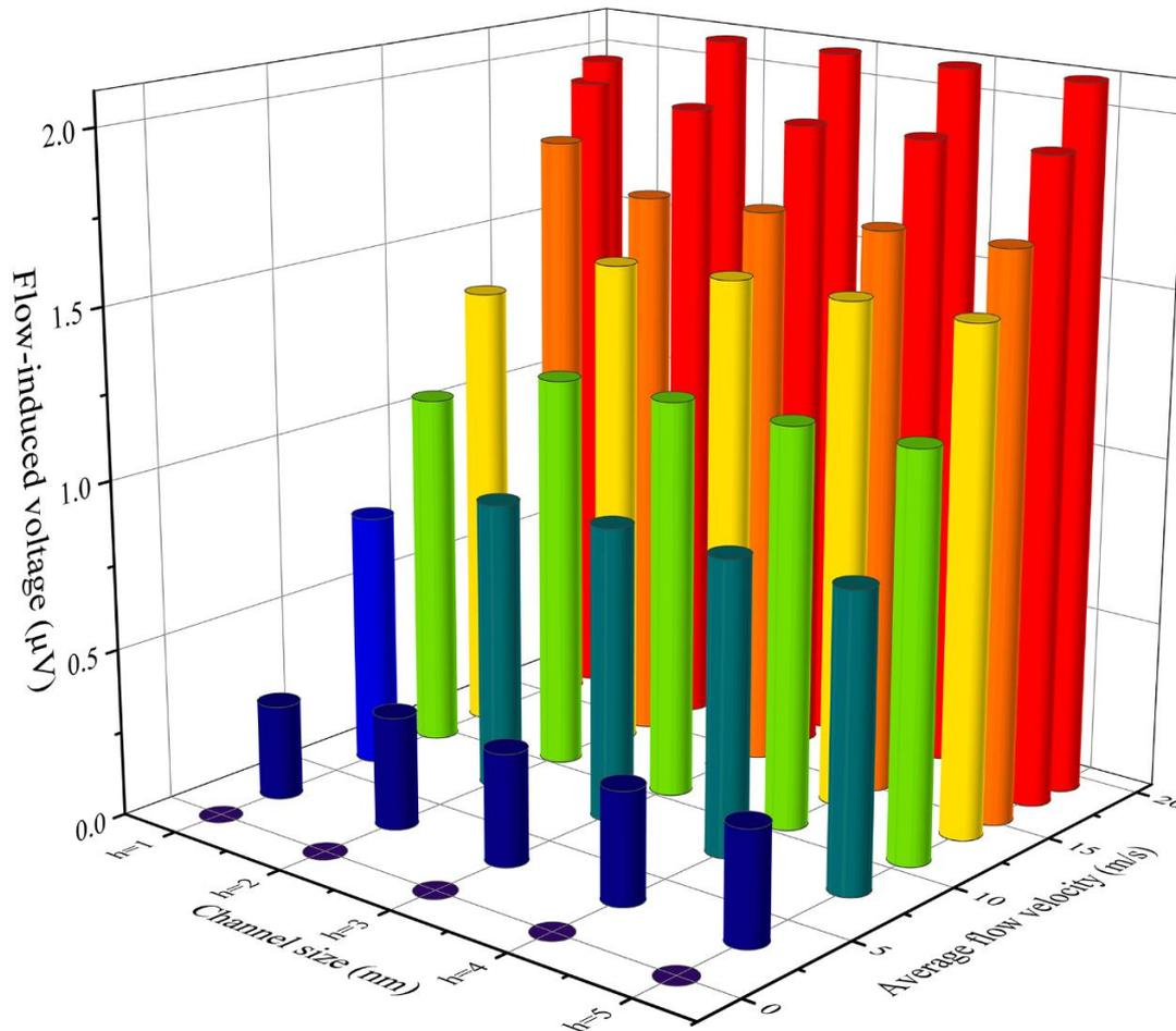
The flow-induced voltage increases from 1.9 to 2.1  $\mu\text{V}$  as the graphene nano-channel size increases from 1 to 5 nm, tending toward saturation as average flow velocity increases.
