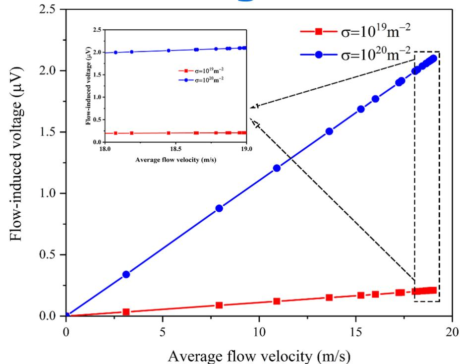
The flow-induced voltages is about 2.1  $\mu\text{V}$  and tends to saturation as average flow velocity increases.
