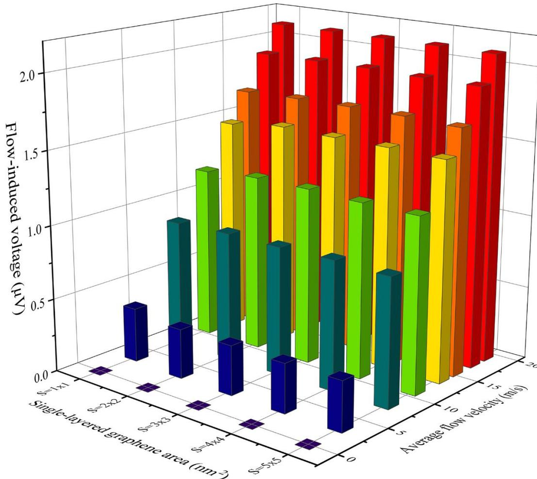
The flow-induced voltage decreases from 2.3 to 2.1  $\mu\text{V}$  as the graphene area increases from 1 to 25  $\text{nm}^2$ , then tending to saturation as average flow velocity increases.
