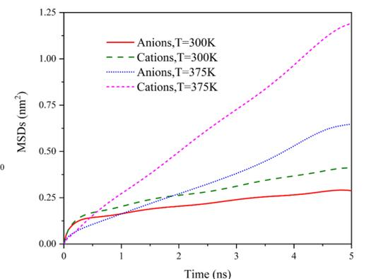
The flow-induced voltage (2.4 μV) has a significant increase at T = 375 K which could be attributed by the change of viscosity (mean square displacements).
