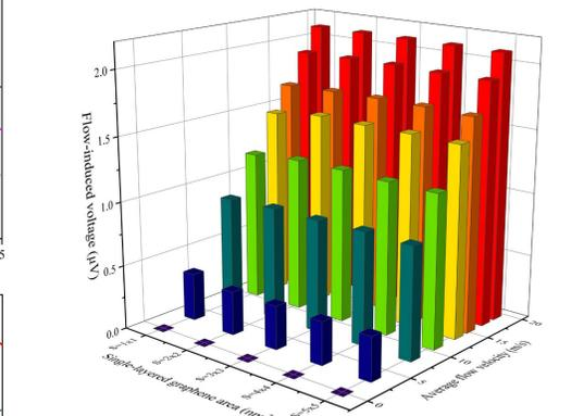
The flow-induced voltage decreases from 2.3 to 2.1 μV as the graphene area increases from 1 to 25 nm<sup>2</sup> and then tends to saturation, which is quantified by the mean square displacements of cations and anions.
