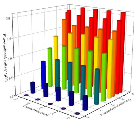
The flow-induced voltage increases from 1.9 to 2.1 μV as the graphene nano-channel size increases from 1 to 5 nm and then tends to saturation, which is quantified by the radial distribution function of ions.
