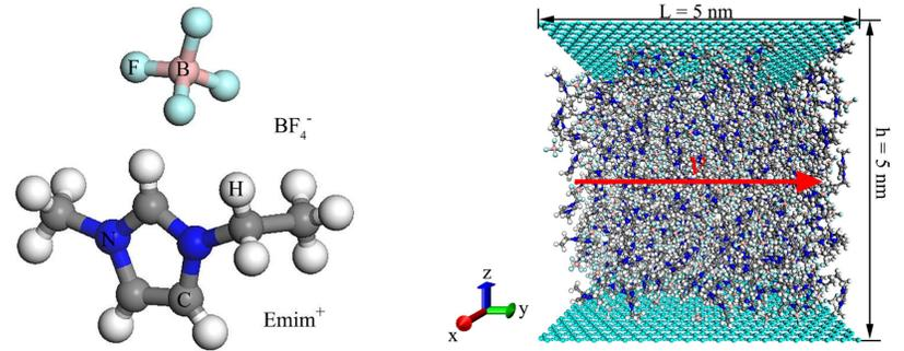
The simulated model is comprised of 1-ethyl-3-methylimidazolium tetrafluoroborate ([Emim][BF<sub>4</sub>]) ILs and graphene channel. After the simulated systems reach equilibration, a series of accelerations from 0.001 to 0.2 nm ps<sup>-2</sup> are applied in systems along y direction.
